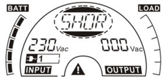
■ Figure 6.5 The Fault mode
